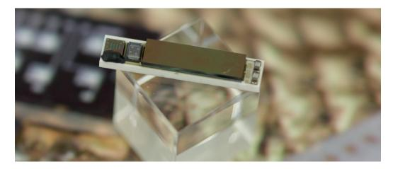
Overall system including pressure and acceleration sensor with a length of about 15 mm and a diameter of about 3 mm.
